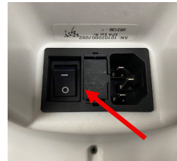
on/off switch - = on O = off
