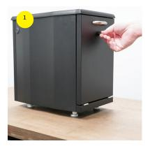
Turn thumbscrew on front panel 90 degrees counterclockwise to open.
