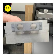
Align cover plate to fit over back end of both bulbs and replace.
