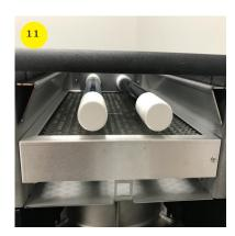
Ensure both UV-A bulbs are properly seated into bulb sockets.
