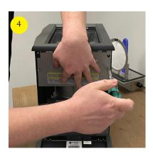
Using a Philips screwdriver, emove two screws on cover plate.
