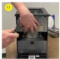
Tighten left and right screws on cover plate.
