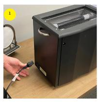
First, ensure power cord is removed from the Sentry device.
