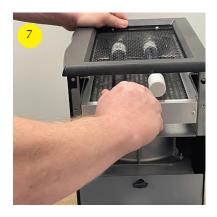
Pull old bulb straight out of socket.
