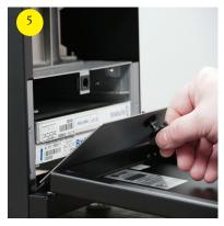
Check compartment for loose debris.
