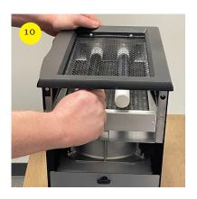
Push UV-A bulbs firmly into place in bulb sockets.
