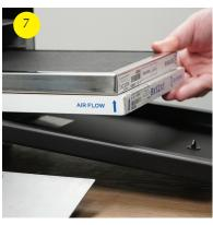
Replace carbon filter on top of the MERV 11 filter.
