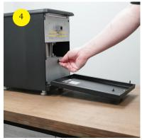
Turn knob on filter compartment 90 degrees counterclockwise to access
