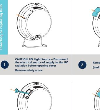
Remove bulb cover (and bulb if already inserted)
