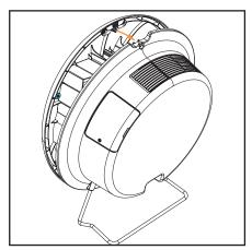
To put the cover back on, position the top and bottom pins over the slots. Let the magnets reengage. Fasten the safety screws.
