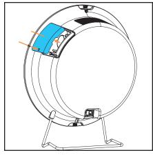
Replace bulb cover and fasten the screw.
