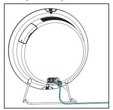
The power cord and power switch are located on the back of the device.
