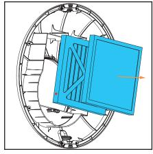
Remove the old filters and replace with new ones\*.
