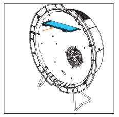
Hold tabs and insert the Sail flat and horizontally into the slot near the top of the device.
