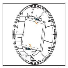
Turn tabs 90 degrees to secure the new filters in place.
