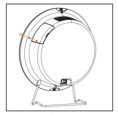
Remove the safety screw on the bulb cover, using the "L" shaped Torx Tool.
