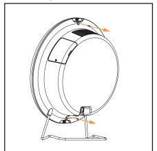
Remove the safety screws at the top and bottom.
