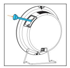
Align the 4 pins to the female socket connectors and insert the new bulb.
