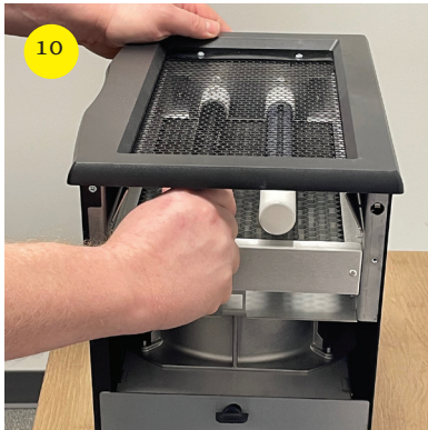
10 Push UV-A bulbs firmly into place in bulb sockets.
