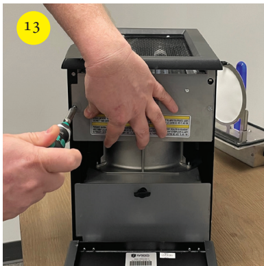
13 Tighten left and right screws on cover plate.
