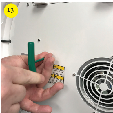
Make sure security screw is tightened all the way.
