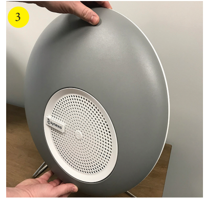
Grab recess and pull top and bottom of cover to disengage magnets.
