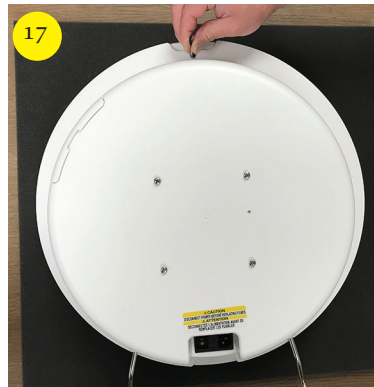
Tighten top safety screw.
