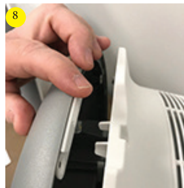
Position top pin over slot. Let magnet re-engage. Fasten safety screws.
