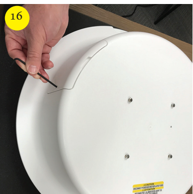
Tighten UV bulb cover safety screw.
